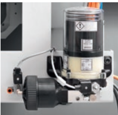
Automatic lubrication boring head BHZ 29 2L.
