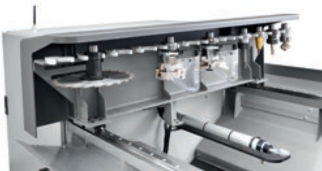
Rack tool magazine with 12 places, with integrated pick-up.
